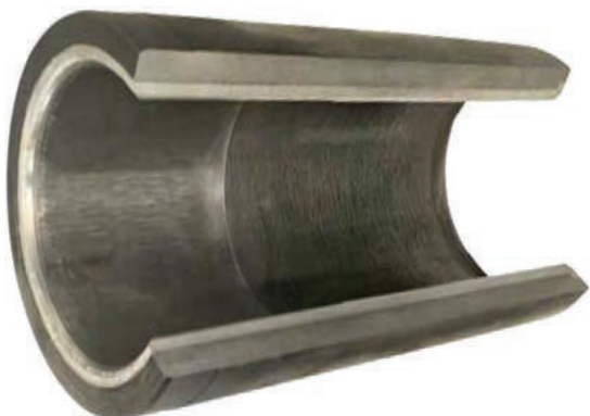
Figure 6. Appearance of a surfaced bushing of 160 mm diameter
