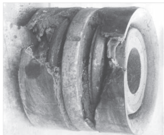
Figure 8. Appearance of the piston with rubber collars after studying a bushing deposited with powder of N75Kh15S4R4 alloy
